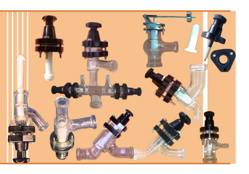
This section covers a diverse range of valves. Each valve made of borosilicate glass body and a PTFE valve bellow, ensuring that the process fluid only comes into contact with glass and PTFE. The borosilicate glass body also allows for visual inspection of the valve's operation.
